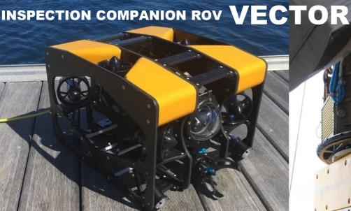
The Vector is a **deepwater** observation system. It consists of the fly-out ROV and a Tether Management System (TMS) with 60m of tether cable.
